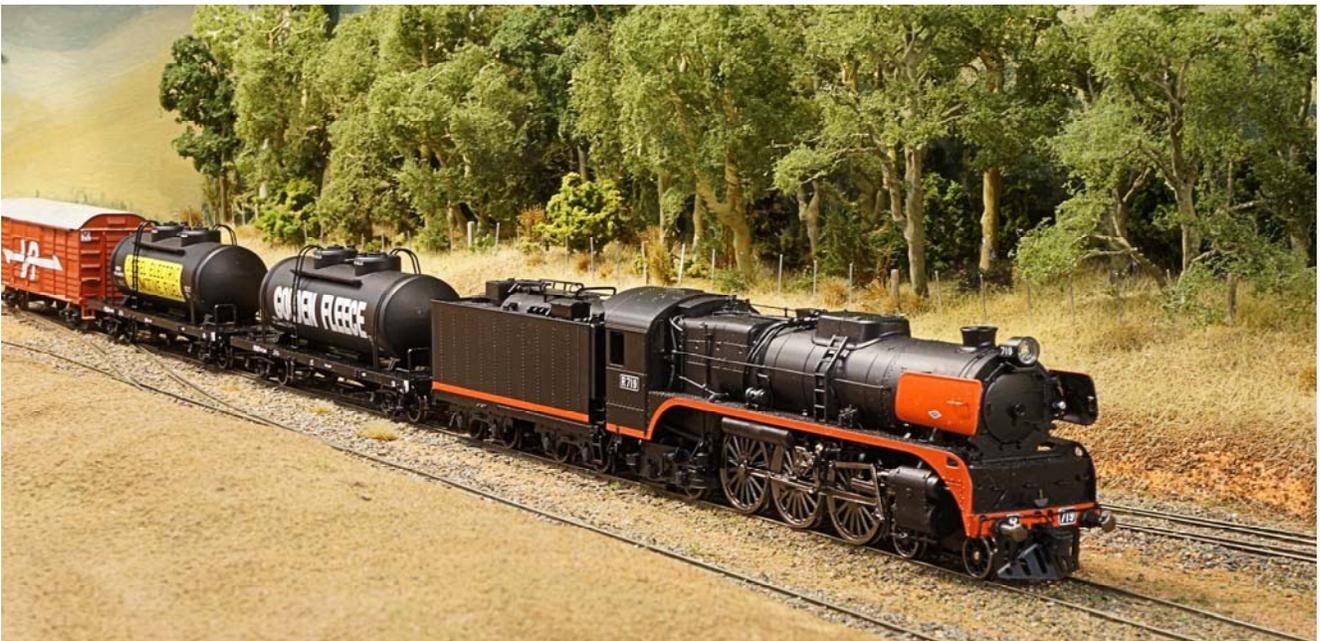
Oil burning R 719 at the head of a short goods which includes a pair of bogie oil tank wagons.
